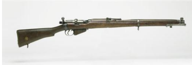
A Lee Enfield .303 bolt action rifle. The standard rifle for the British army in WWI. You could fire it 11 times without reloading. (It could carry 10 rounds (bullets) in its magazine and could keep 1 round in the gun ('up the spout').)
